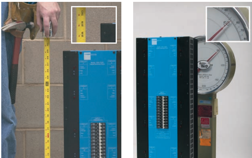
The SSD-12/20 is 29 inches tall and weighs 53 pounds.
