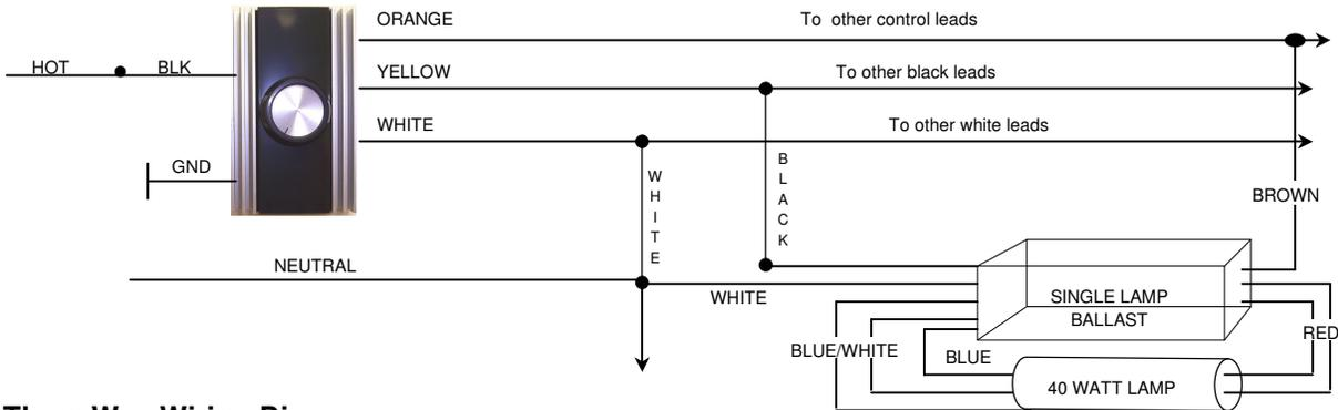
**Three Way Wiring Diagram**
