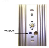
Turn control switch pot full clockwise; with a small screwdriver, slowly turn trimpot (clockwise to <u>decrease</u> / counterclockwise to <u>increase</u>) to the desired R.P.M.
